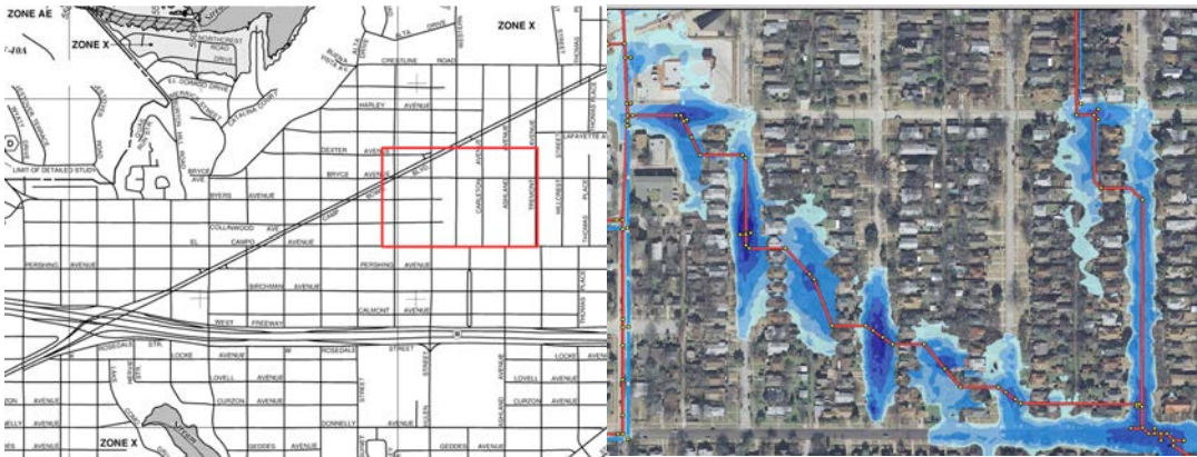
FIGURE 36. MAP ON LEFT IS A FIRM FOR A NEIGHBORHOOD IN A TEXAS COMMUNITY. THE GRAY SHADING INDICATES THE SFHA IN THAT AREA. THE RED BOX IDENTIFIES THE LOCATION OF THE AREA SHOWN IN THE RIGHT MAP WHERE, DUE TO PROBLEMS WITH THE LOCAL DRAINAGE, THE AREAS SHOWN IN BLUE ARE SUBJECT TO URBAN FLOODING BUT NOT REFLECTED ON THE FIRM. SOURCE: THE ASSOCIATION OF STATE FLOODPLAIN MANAGERS ANNUAL CONFERENCE, 2018.
