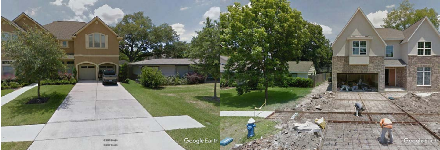
FIGURE 20. LARGE HOMES REPLACE SMALLER HOMES, INCREASING RUNOFF FROM ROOFS AND DRIVEWAYS (HOUSTON). SOURCE: GOOGLE EARTH.
